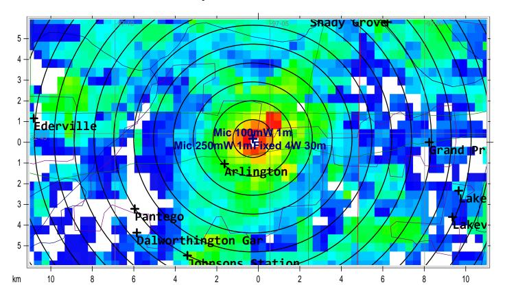
Receive Signal Level in dBm with COR of RX antenna at 2 meters.
